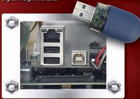
The 825 Spectrum's USB drive supports data transfer, USB QWERTY keyboards, and Cardinal-supported printers.
