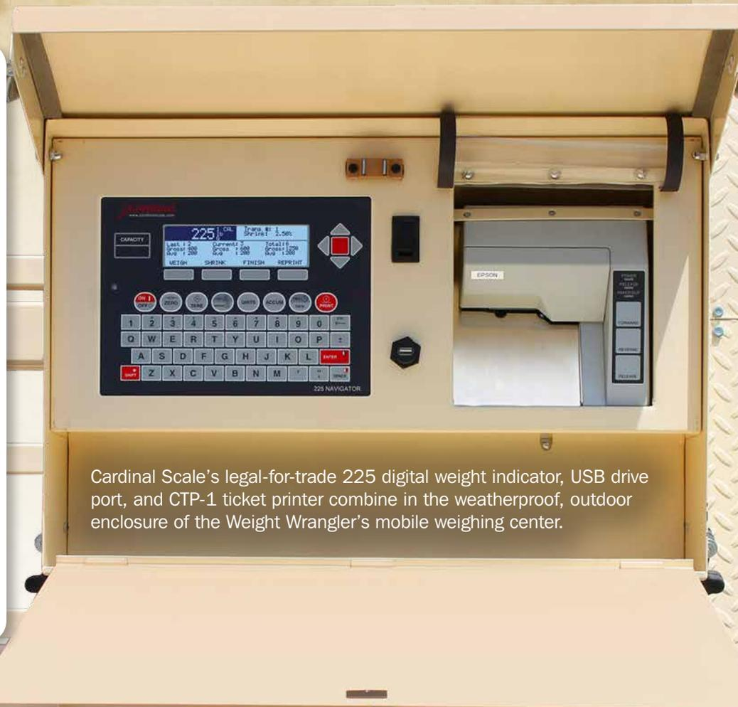
Cardinal Scale's legal-for-trade 225 digital weight indicator, USB drive port, and CTP-1 ticket printer combine in the weatherproof, outdoor enclosure of the Weight Wrangler's mobile weighing center.
